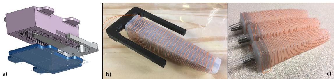
Figure 3.14: RBO-Style Fiber Reinforced Fingers: (a) and (b) Finger mold, modified for injection, (c) Finger with fiber reinforcement added after assembly with strain limiting layer, (d) Finger with strain limiting layer added after fiber reinforcement, (e) Delamination problems
