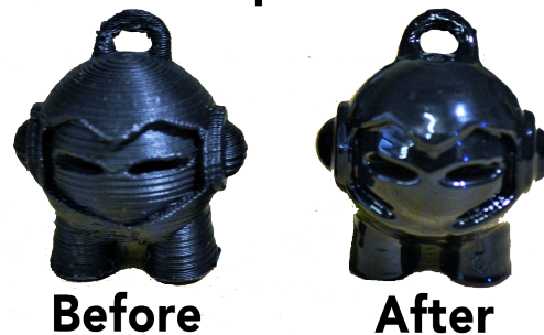
Figure 2.18: Effects of acetone smoothing
