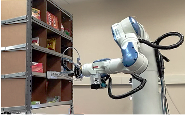
Fig. 2. A Motoman SDA10F robot carrying the UniGripper tool and an Amazon-Kiva Pod stocked with objects.
